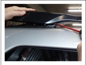
2. If factory rails are fitted, carefully pry off the six plastic shrouds using a sharp screw driver.
