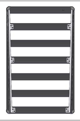
14. Flip the blade brackets over so they are upside down and carefully place on top of the BASERACK. When doing so ensure the M8 studs in the stud plates go through the slots. Then secure the blade brackets to the BASERACK using M8 flat washers and nyloc nuts.
