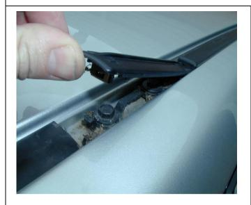
1. Remove the six plastic plugs or factory rails that run along the recessed channel in the roof, exposing the bolts and pressed brackets.
