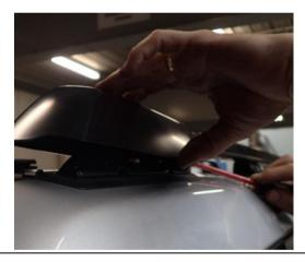
3. Remove the bolts, washers and bracket. Lift off roof rails if fitted.
